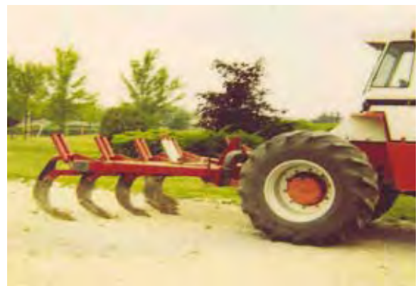
Fig. 7. One of several variations of an agricultural ripper. This unit has long, rugged shanks mounted on a steel V-frame for deep, aggressive fracturing through Phase 1.
