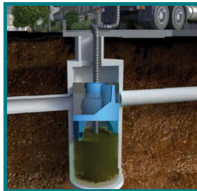
Fig 3. Maintenance is done with a vector truck
