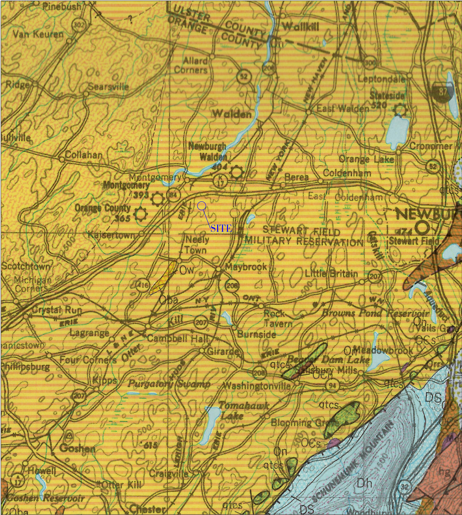
Approximate location of the project site, shown on part of the Bedrock Geologic Map of New York (1970.) The site is in the middle of a wide belt of Ordovician-age sedimentary bedrock consisting mostly of gray siltstone, shale and greywacke sandstone. The bedrock at the site is shown as Normanskill Formation (yellow with red stripes, symbol On,) which is the oldest member of this Ordovician sequence, with the Austin Glen Formation (yellow with red stipple) overlying it, which in turn lies below the Quassaic quartzite. These units form the bedrock of most of the Wallkill River valley. Older Ordovician carbonate rocks, the Wappinger Dolostone (symbol Ow) and the Balmville Limestone (Oba) outcrop about a mile south of the site, on the opposite side of the railroad; that bedrock was faulted into place and overlies the shale.
