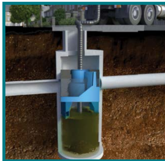
Fig 3. Maintenance is done with a vector truck
