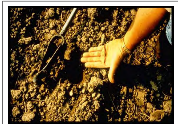
Fig. 5. Augered from a depth of 19 inches below the surface of the replaced topsoil, this subsoil sample was hand rolled to a 1/8-inch diameter. The test shows the soil at this site stretches out too far without crumbling; it indicates the material is in a plastic state of consistence, too wet for final decompaction (deep subsoiling) at this time.
