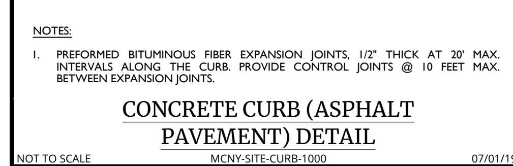
CONCRETE CURB DETAIL
