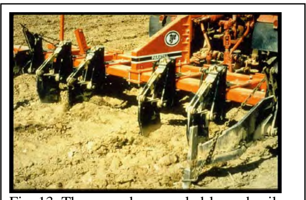
Fig. 13. The same deep, angled-leg subsoiler shown in Fig. 7 is engaged at maximum depth for Phase 2, decompaction (deep soiling), of the replaced topsoil and the upper subsoil materials.
