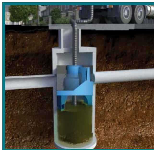
Fig 3. Maintenance is done with a vactor truck
