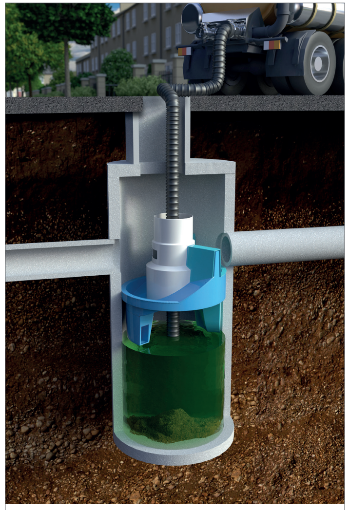
Fig.4 Floatables are removed with a vactor hose
